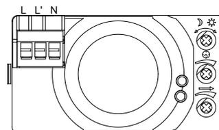
Connecter N, L à l'alimentation; Connect N, L' with load.
