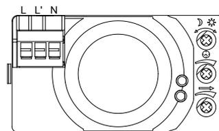
Connect N, L with power; Connect N, L' with load.
